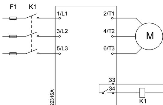
*Soft starter installed with a shunt relay and circuit breaker*
